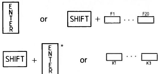
If the keyboard is locked, data communication can **only** be initiated with the keys **K1**, **K2**, **K3**.
