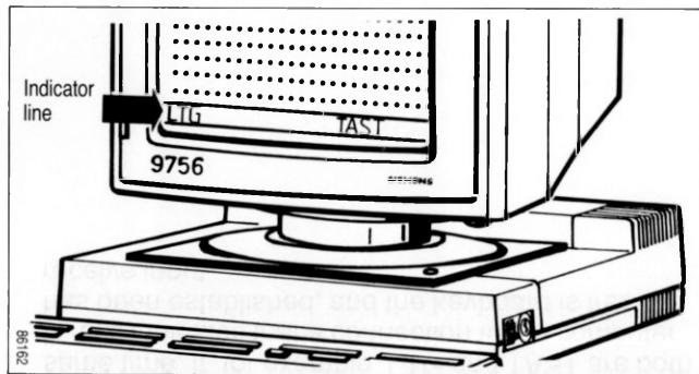
The device indicator line is the separate, bottom line of the screen.
