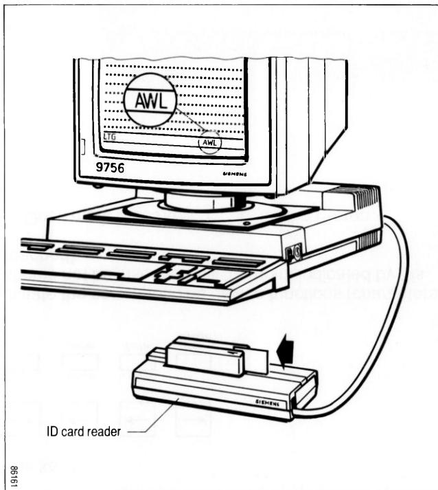
A 9007-97 "pull-through" ID card reader can be connected to the data display terminal. This requires the installation of an adapter set in one of the plug-in locations in the control unit.
